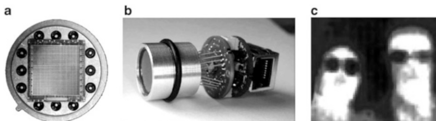
Fig. 15.25 Thermopile thermal-imaging sensor. Sensing surface (a); imaging module (b); example of a thermal image (c) (Courtesy of Heimann Sensors GMBH)
