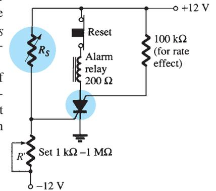
FIG. 17.19 Alarm circuit.
