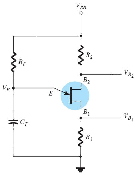
FIG. 14.37 Basic unijunction oscillator circuit.
