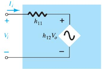
FIG. 5.94 Hybrid input equivalent circuit.
