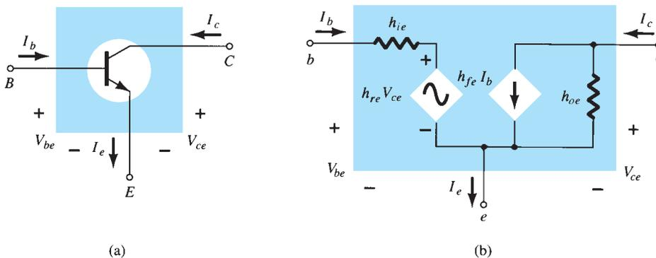
FIG. 5.97 Common-emitter configuration: (a) graphical symbol; (b) hybrid equivalent circuit.
