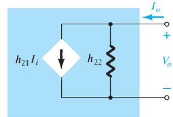
FIG. 5.95 Hybrid output equivalent circuit.
