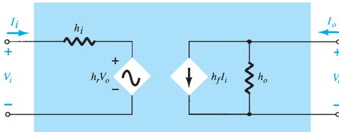
FIG. 5.96 Complete hybrid equivalent circuit.
